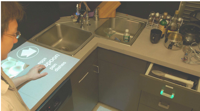
Figure 6. Three modalities for location-sensitive display: image, text and colored illumination.
