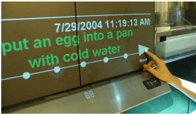
Figure 2. A step-by-step recipe with camera-based touch interface.
