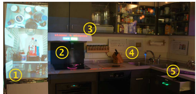
Figure 1. Augmented Reality Kitchen: information projection on the refrigerator (1), the range (2), the cabinet (3), the faucet(4) and drawers(5).
