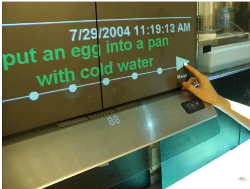
Figure 3. Virtual Recipe projected onto the cabinets and Rangefinder temperature on the hood.
